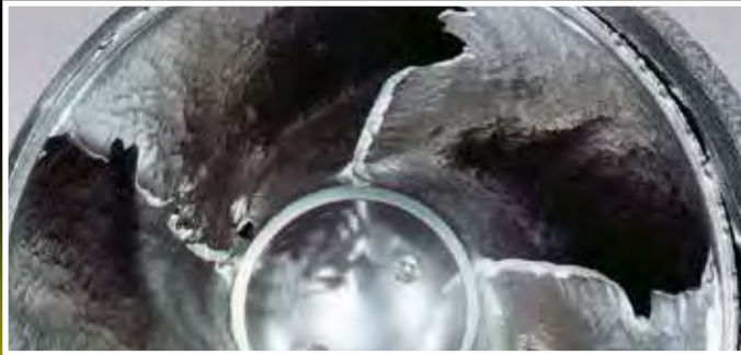
Impeller made of Duplex Stainless Steel Heavy wear after 11,000 operating hours
