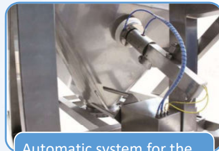
Automatic system for the Vibrator activation
